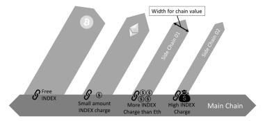
Figure 4.9: Fee Mechanism of Indexing aelf Side Chains
